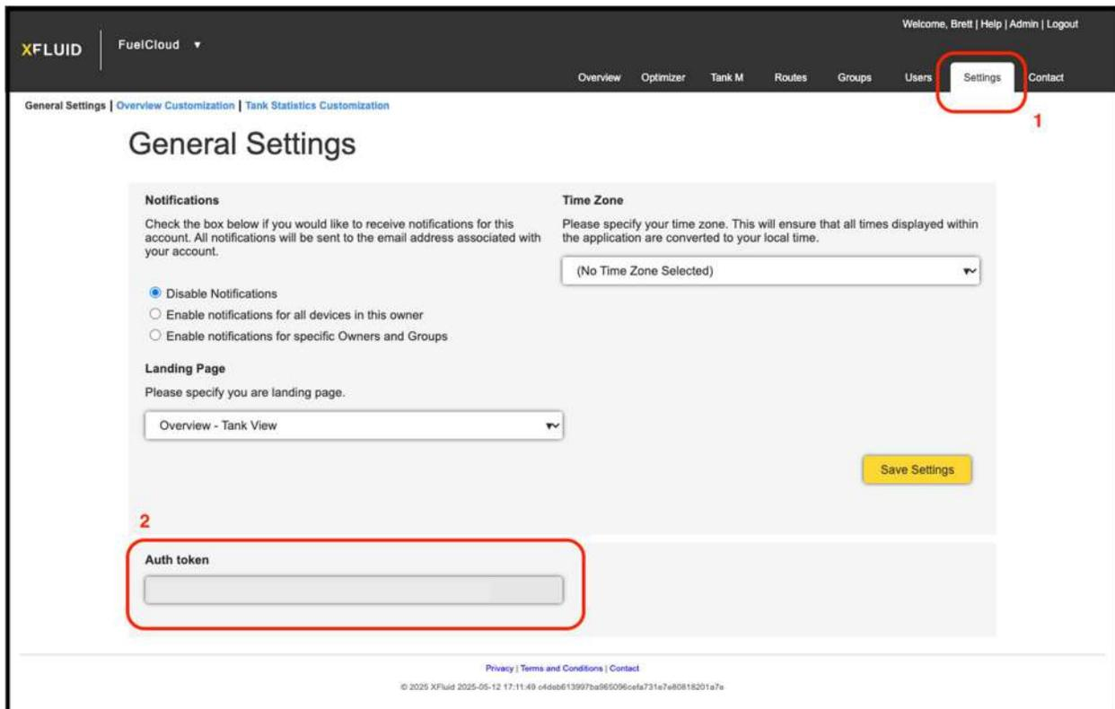
2. On Anova XFluid, you will also need to set up a data feed
